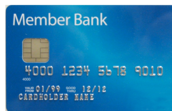
Figure 1: Contact EMV Smart Card
