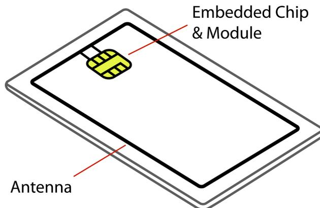
**Figure 6. Dual-Interface Smart Card**
