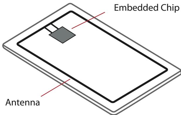
**Figure 5. Contactless Card**
