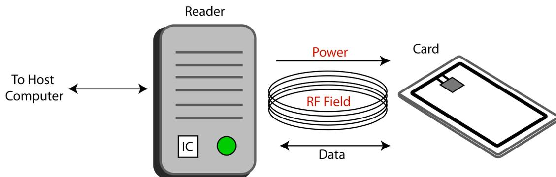
**Figure 4. Contactless Smart Card in RF Field**
