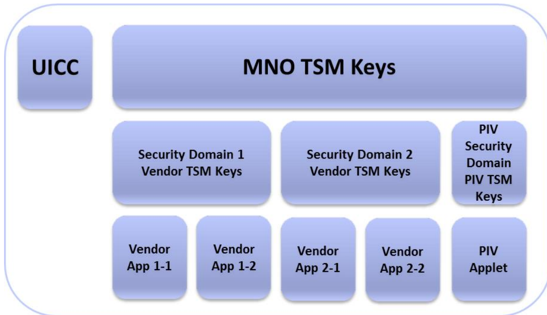
Figure 2. Establishment of a Dedicated, Separate Security Domain for the PIV Applet
