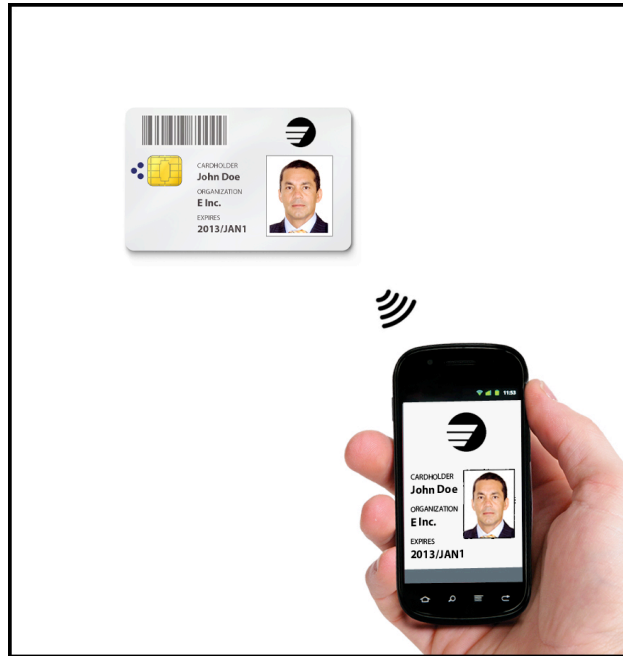
Figure 4. NFC-Enabled Mobile Phone Used as a Reader
