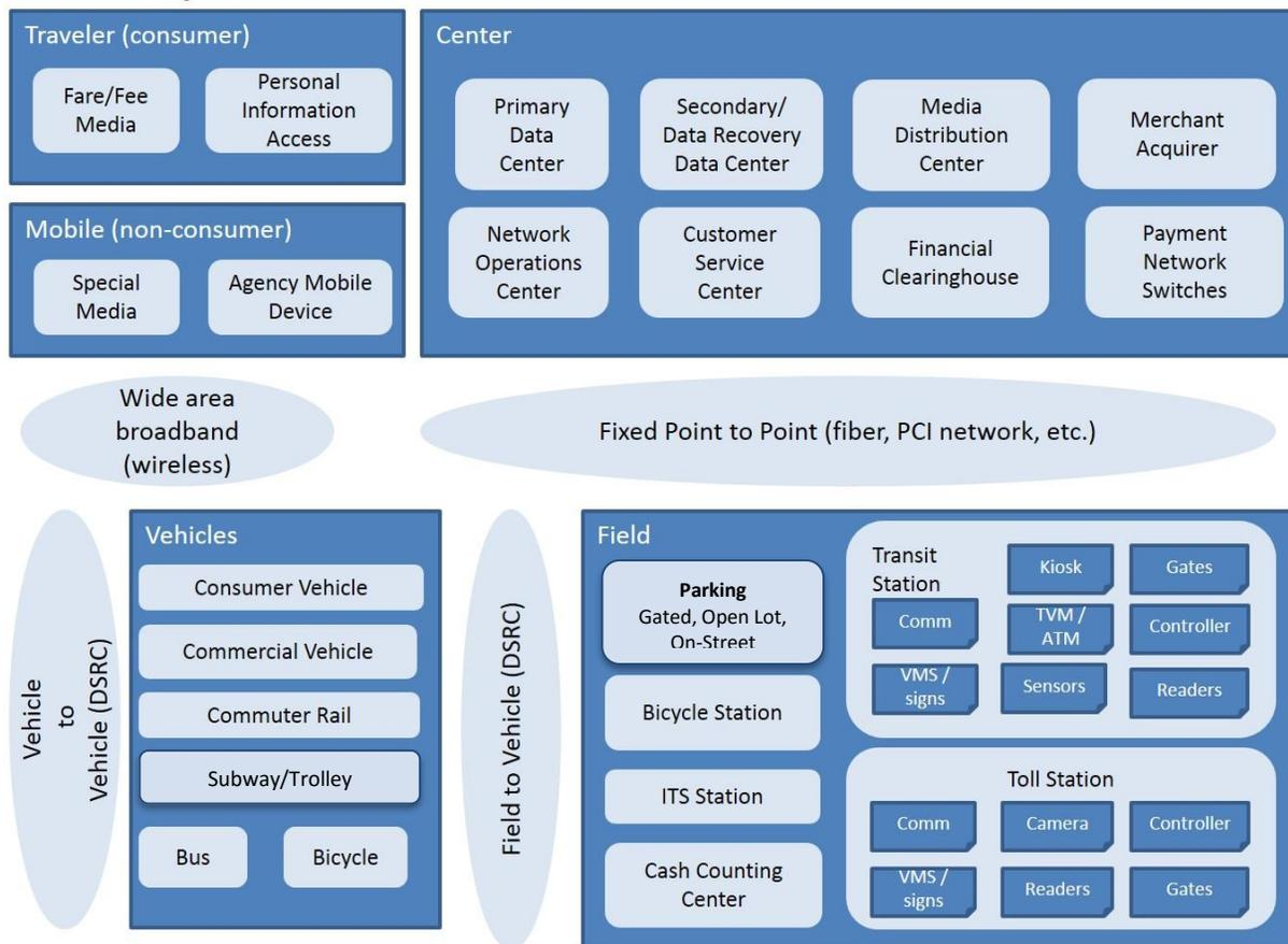
Figure 10: Technology (Template) Layer (Draft Version)
